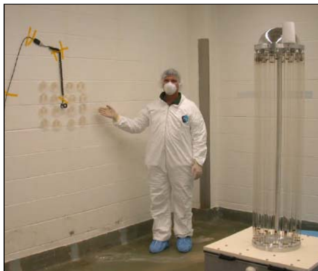
TRU-D prototype in test room with sensors and contaminated test plates.
