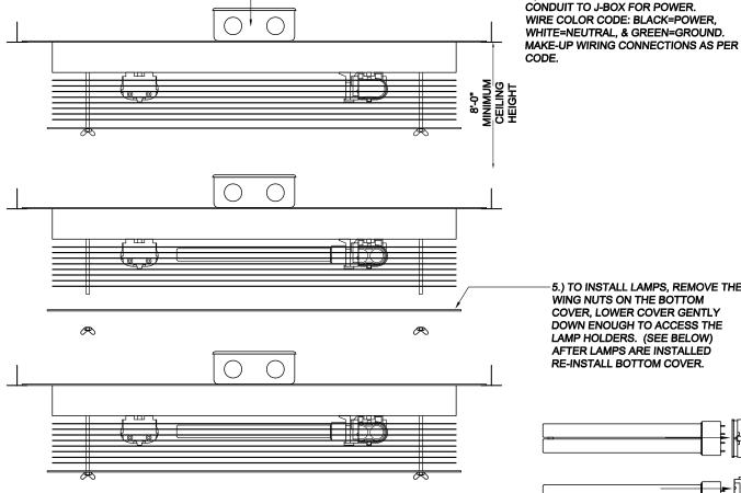
5.) TO INSTALL LAMPS, REMOVE THE WING NUTS ON THE BOTTOM COVER, LOWER COVER GENTLY DOWN ENOUGH TO ACCESS THE LAMP HOLDERS. (SEE BELOW) AFTER LAMPS ARE INSTALLED RE-INSTALL BOTTOM COVER.
