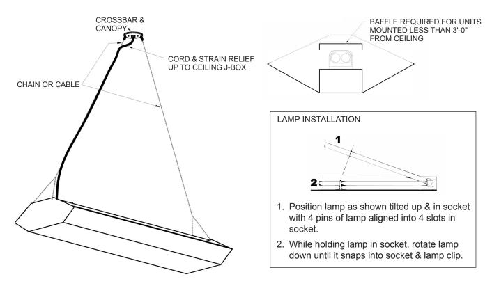
If ceiling height is lower than 10'-0" or if fixture is mounted less than 3'-0" from ceiling, baffle is required. Installation & removal of baffle is done so by screwing or unscrewing screws from each end of baffle. Lamp fixture, read caution, re-energize fixture.
